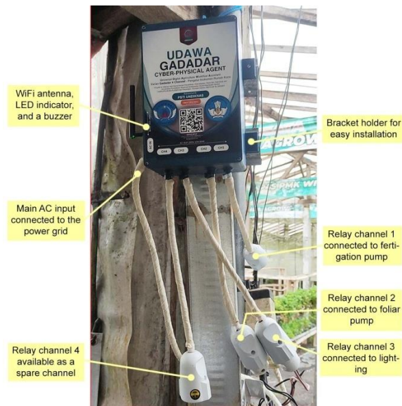
Figure 7. The installation of the UDAWA Gadadar agent at one of the strawberry greenhouse, showing three greenhouse instruments connected to the universal plug
