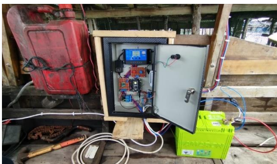
Figure 5. Implementation of the Overall Hardware Circuit in the Automatic Water Drainage System at the Pump
