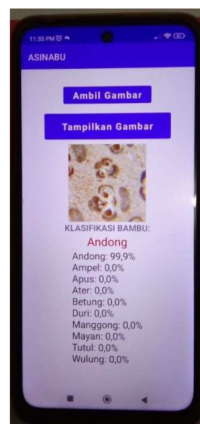
Figure 10. Asinabu Photo detects Andong bamboo with 99.9% accuracy on the Xiaomi Redmi 5G cellphone
