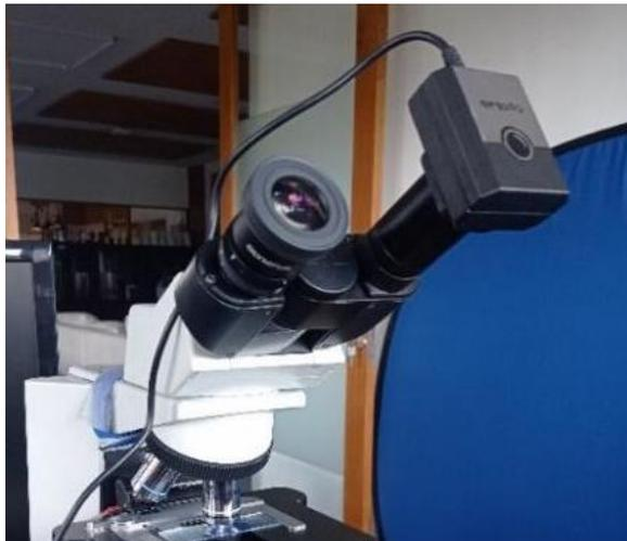
Figure 13. Camera position on the microscope lens
