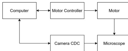
Figure 2. Microscope workflow
