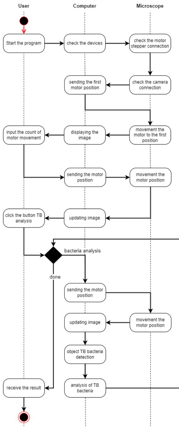
Figure 8. Automatic microscopic shift and shooting workflow
