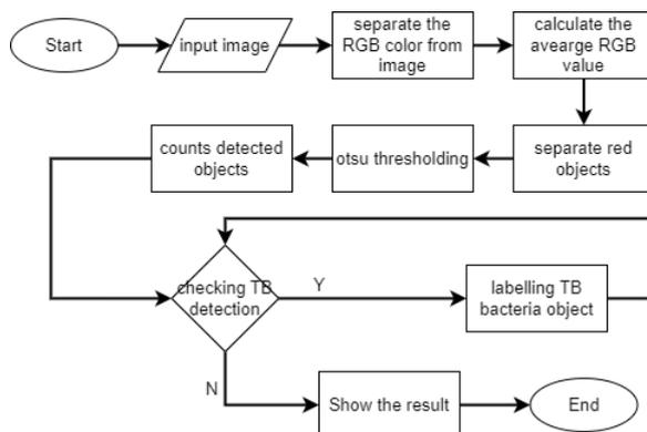
Figure 9. TB bacteria detection flow
