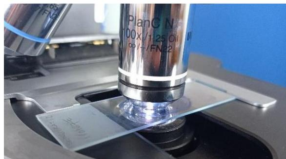
Figure 6. Mounting prepare on a 100x magnification lens
