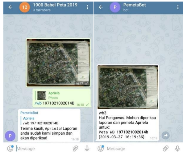
Figure 5. Field Officer is reporting the WB Map via Group (Left). Telegram Bot sends a report message to the Supervisor for review (Right).
