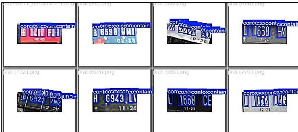
Figure 9. Sample Characters Detection on the Plate
