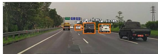
Figure 4. Object Detection in Dashcam (Smartphone) [33].
