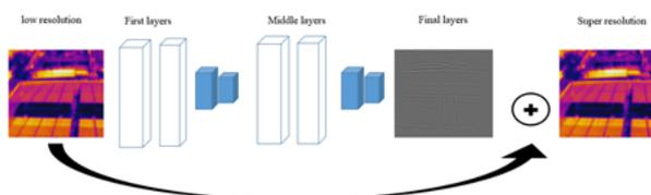
Figure 4 The architecture network of proposed network
