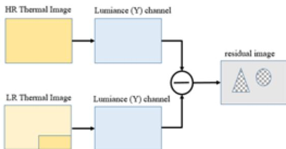
Figure 5. The block diagram of generating dataset
